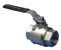
2 PIECE BALL VALVE Firesafe Certified Lockable lever operated 316 Stainless Steel Full Bore, PTFE seats 2000 PSI 8mm-25mm NPT 1500psi 32 to 50mm NPT 1000psi 80 to 100mm NPT
