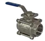
3 PIECE BALL VALVE ISO DIRECT MOUNT 316 Stainless Steel Full Bore Lockable lever operated PTFE seats 8mm to 100mm BSP 1000 PSI
