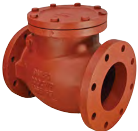
CAST IRON SWING CHECK VALVE Bronze seat Flange AS2129 Table E 50mm to 300mm Undrilled available
