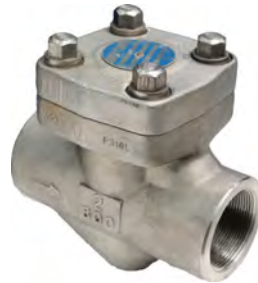
PISTON CHECK VALVE API602 316 Stainless Steel Stellite seat CLASS 800 (2000psi) NPT or socket weld 15mm to 50mm
