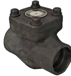
PISTON CHECK VALVE API 602 A105N Stellite seats CLASS 800 (2000psi) NPT or socket weld 15mm to 50mm
