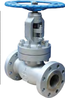
FLANGED GLOBE VALVE ANSI 150 or ANSI 300 316 Body, STELLITE seat OS&Y Graphite Packing Spiral Wound Gasket 15mm to 300mm
