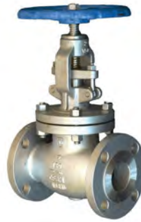
FLANGED GLOBE VALVE ANSI 150 or ANSI 300 316 Body, STELLITE seat OS&Y Graphite Packing Spiral Wound Gasket 15mm to 300mm
