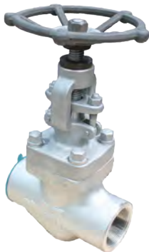
GLOBE VALVE API 602 316L Stainless Steel CLASS 800 (2000psi) Stellite seats 15mm to 50mm NPT or socket weld
