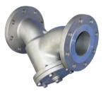
**YST--** 150 - 300 - 600 FLANGED Y STRAINER ANSI 150 - 300 - 600 316 Stainless Steel Integral drain plug 15mm to 300mm Available undrilled
