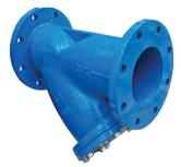
CI YST CAST IRON Y STRAINER FBE Coated S/S Screen Flanged AS2129 Table E 50mm to 600mm 100mm & 250mm available Table D
