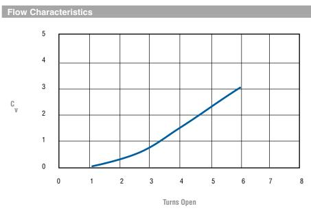
$^{3/\!8}\text{-inch}$  [9.5 mm] orifice,  $C_V$  3.0 maximum
