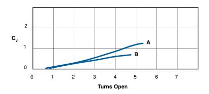
A =  $^{1/4}$ -inch [6.4 mm] orifice, valve C\_V 1.4 maximum B =  $^{3/16}$ -inch [4.8 mm] orifice, valve C\_V .83 maximum
