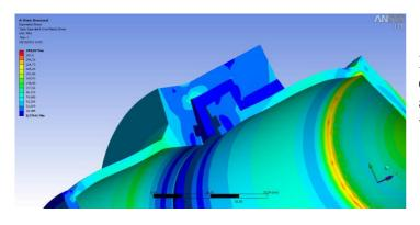
In addition, the design phase involves a finite element analysis to identify the most stressed areas and to control the heat loss during welding operations.
