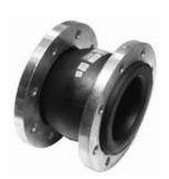
Site engineers or installers to ensure Lateral Angular Deformation is not to exceed 15 Degrees on sizes up to 600mm on standard single sphere rubber joints, along with design Axial extension and Compression compliances. Always ensure the material grades suit the application.
