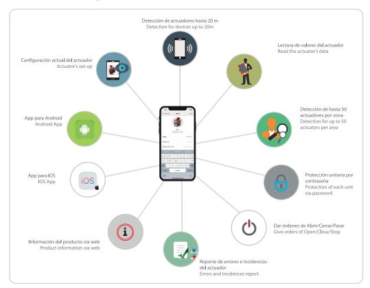
We have introduced the BLUETOOTH communication system in our actuators, in order to communicate with our actuators, from any IOS or ANDROID devices.
