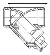
Strainers offer a vital safeguard against rust, scale and dirt installed In steam, water or chemical pipework systems. They protect expensive and sensitive equipment such as steam traps, pressure reducing and control valves. By protecting equipment they reduce costly production down times through unnecessary maintenance.
