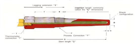
A thermowell is a cylindrical fitting used to protect temperature sensors installed when measuring liquid such as in the production of beer, the thermowell protects the thermometer when measuring the temperature as well as protects the liquid from contamination. The thermowell acts as a barrier between the device measuring temperature and the liquid as well as the liquid from the outside air.
