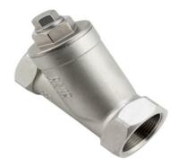
Strainers offer a vital safeguard against rust, scale and dirt installed In steam, water or chemical pipework systems. They protect expensive and sensitive equipment such as steam traps, pressure reducing and control valves. By protecting equipment they reduce costly production down times through unnecessary maintenance. They require regular cleaning hence the blowdown plug for fitting a drain valve as below.
