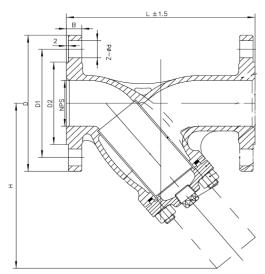
Screen mesh is SUS 316 SS material with perforation 1.mm to 1.6mm Mesh interlining options of 60 and 100 mesh.
